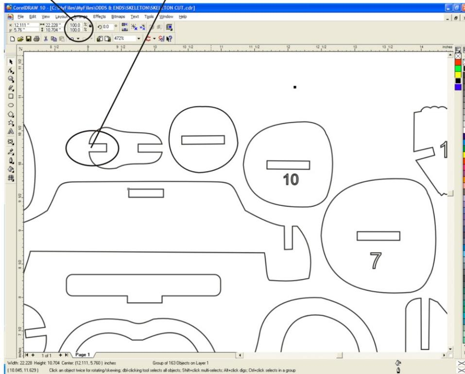
Once you resize the design, I like to use the rectangle tool (F6) to draw a small box to check the slot size.
